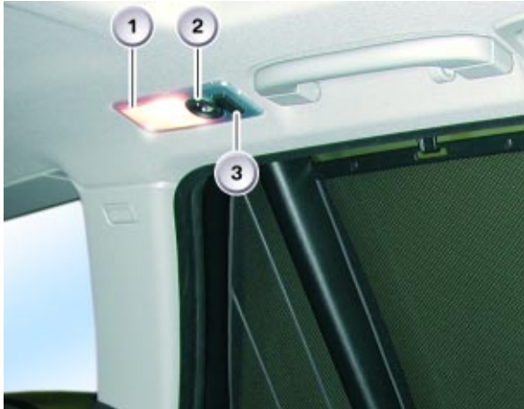
Installation location of rear interior light on driver's side (passenger side symmetrical)
